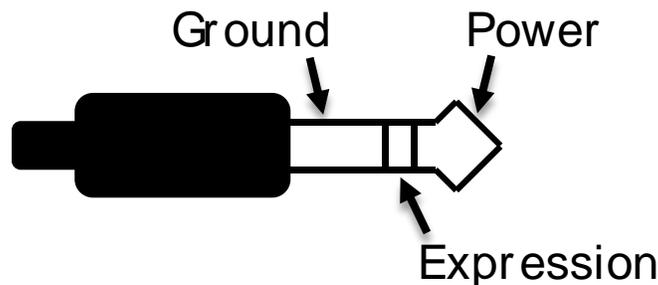
Expression pedals with TS (Tip Sleeve) plugs will not work correctly with the CONTROL INPUT of the Ventris. For proper operation, the configuration steps in the next section must be followed when using any expression pedal, whether from a third party or from Source Audio.
