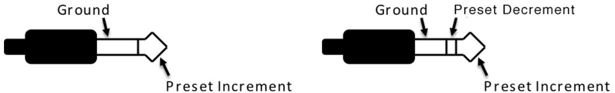
With the Neuro Desktop Editor, it is also possible to assign a number of different control functions to an external switch. Go to the Neuro Desktop [Hardware Options](#) section for instructions on assigning alternate control options to an external dual or single external switch.
