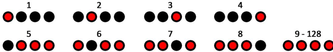
*Note: when using a MIDI controller to select a preset outside of the normal bank (presets 1 to 4) or extended bank (presets 5 to 8), then all 4 PRESET LEDs will be lit, indicating that a preset in the range between 9 and 128 is active. For details on preset editing and saving, see the next section.*
