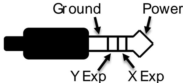
Third party expression pedals can be connected to the CONTROL INPUT as well, as long as they have a 3.5 mm (1/8") TRS (Tip Ring Sleeve) plug with power on the tip, expression (the wiper of the potentiometer) on the ring, and ground on the sleeve, as seen in the diagram below.
