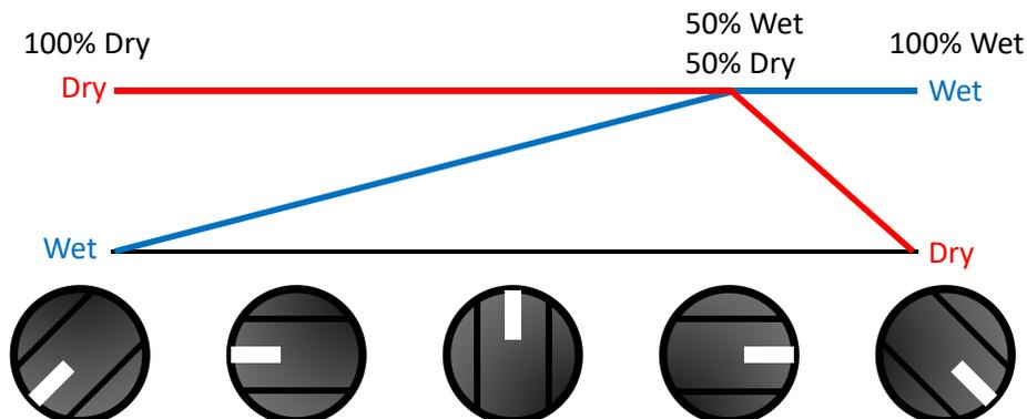
Please note that when the A/B Reverb Toggle Switch is set to the A+B position, the function of MIX and CONTROL 1 & 2 change. In A+B mode the CONTROL 1 knob adjusts the wet level of reverb A, CONTROL 2 adjusts the wet level of reverb B, and the MIX knobs adjusts the level of the dry signal.
