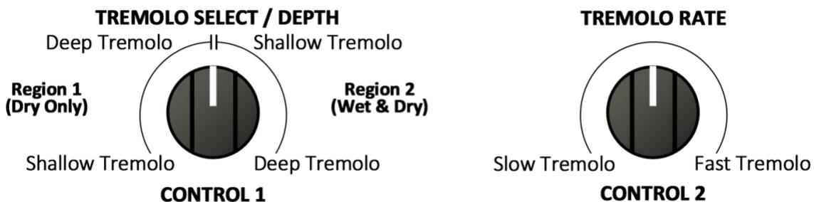
**OPTION FOOTSWITCH (TAPPING):** *Tremolo Rate* – Functions like a traditional tap tempo switch to set the speed of the tremolo effect. Tapping the OPTION footswitch in time with the band will
