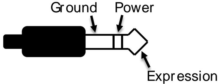
Please note, expression pedals with TS (Tip Sleeve) plugs will not work correctly with the expression input (PEDAL IN jack) of the Ventriss. Also, the resistance of the expression pedal is not critical. Pedal calibration is done automatically when a new external control mapping is created.
