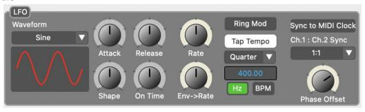
The LFO utilized by the Ultrawave's multi-tremolo can be either a sine wave or a user-defined "Attack/Release" wave. (The single tremolo uses a standard sine wave only.)
