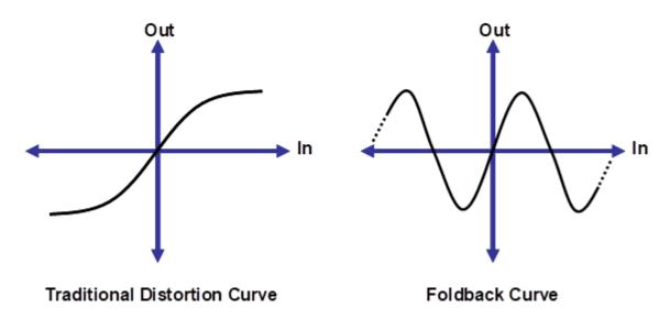
Foldback distortion is one of the many distortion curve options on the Ultrawave. It is worth some background because they are not commonly found in effect pedals. In traditional distortion, as the input signal voltage rises, the output voltage also rises, but begins to level off and finally pins (or clips) at a maximum value. With a foldback curve, for large enough values of the input, the output will begin to decrease. With more extreme amounts of foldback, after decreasing for a while, the
