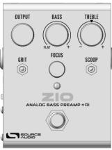
TREBLE – Treble shelving filter centered at 1kHz ranging from -6dB at the min position to +14dB at the max. Note that "flat" is at center of the knob range.
