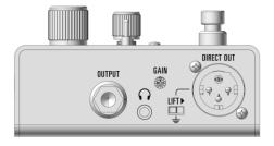
**HEADPHONE OUTPUT** – The headphone output features a high dynamic range, lownoise amplifier that is capable of driving low impedance studio headphones. LIFT – If you're getting "hum" on the direct output, slide the LIFT switch to the right to lift the internal ground connection to the DIRECT OUT XLR jack.
