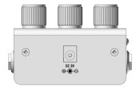
**POWER** – Power the Bass ZIO using the included 9V supply or a pedalboard power supply. Note that the supply should be able to source up to 200mA of current. The unit's high voltage rails and specialized circuit requires more power than typical analog pedals. The high-performance headphone amplifier also adds to the power consumption when in use. Using a higher voltage than 9V is not recommended. Without headphones, the base current draw is around 140mA.
