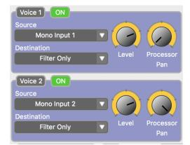
The Spectrum features two standard Voices. Each Voice can receive signal from either Mono Input 1, Mono Input 2, or Stereo Input Mix. Both Voice modules feature the same control set.
