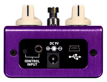
The CONTROL INPUT port opens a variety of external control options, allowing for direct control over many of the Spectrum's parameters. It is an input for the, Source Audio Tap Switch, Source Audio Dual Expression Pedal, or a data port for the Neuro Hub.
