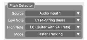
The Spectrum's Pitch Detector is an algorithm that detects the pitch of the connected instrument and uses it as a guide for creating octave effects. In nearly every case the user doesn't need to worry about the response of the Pitch Detector – that said, we do offer some adjustable parameters that refine the Pitch Detector and further decrease latency and improve pitch accuracy. Narrowing the range of notes you expect to play though the Spectrum will help in providing the best possible response.
