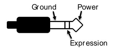
Expression pedals with TS (Tip Sleeve) plugs will not work correctly with the Spectrum.
