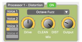
Adds distortion to any of the Standard or Octave Voices. The high harmonic content of added distortion will heavily accentuate the sound of the modulating filters. The Spectrum includes 13 types of distortion, anything from a subtle drive effect to extremely fuzzy Foldback effects.
