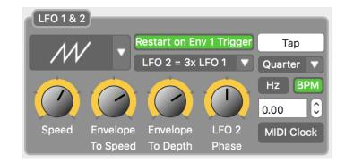
The LFOs (Low Frequency Oscillators) can be set to control the Filter modulation.
