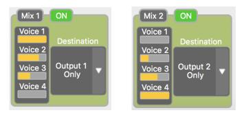
Mix 1 and Mix 2 Blocks: The four meters labeled Voice 1 through 4 monitor the signal ratio routed through Processors 1 & 2. Please note that setting the Destination of *Mix 1* to *Output 1 Only* and *Mix 2* to *Output 2 Only* is necessary in creating stereo effects. Each Voice's position in the stereo spread is set with the Processor Pan control in each of the Voice blocks.
