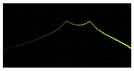
Only a range of frequencies gets through. Higher Q's produce a narrower response.
