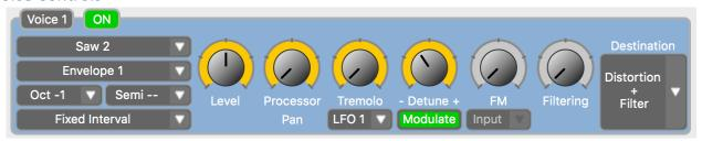
The C4 features four individual Voices. Assign each Voice to any one of the possible options: Sine, Square, or Saw Wave Oscillator, Monophonic Pitch Shifter, Polyphonic Pitch Shifter, or the dry signal routed directly to the envelope filters and/or distortion block. Mix together any combination with each Voice's dedicated Level and Pan Controls. All four Voice modules feature the same control set.
