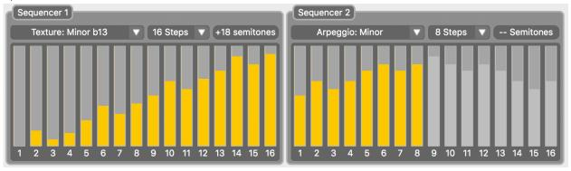
The C4 features two simultaneously running Sequencers. With the Sequencers it is possible to create two note patterns up to 16 steps long. The Sequencers come with 16 different pre-made sequences all of which can be edited into your own custom pattern. Please note that Sequencer 1 responds to Voices assigned to a Source labeled with a "1" (ex. Square 1, Sine 1, Saw 1) and Sequencer 2 responds to Voices assigned to a Source labeled with a "2" (ex. Square 2, Sine 2, Saw 2).
