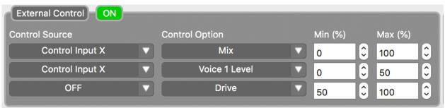
The External Control block is where external expression control is assigned to devices like the Source Audio Dual Expression Pedal, Hot Hand 3 Wireless Controller, and expression devices connected to a Neuro Hub. All external control expression devices connect to the CONTROL INPUT jack on the topside of the pedal with a 1/8" TRRS cable.
