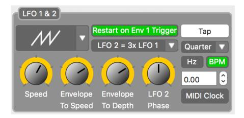
The LFOs (Low Frequency Oscillators) can be set to control the Filter modulation, Sequencer rates, or Tremolo rates (amplitude modulation).
