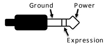
Expression pedals with TS (Tip Sleeve) plugs will not work correctly with the C4.
