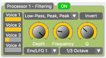
The Filters play a crucial role in developing the character of your preset. Basically a filter boosts or cuts certain segments of a sound's frequency spectrum. Modulating these filters (a.k.a moving them up and down over the signal) creates an effect similar to many of the sounds we hear in the physical world (for example the sound of an instrument being struck or that of a human voice). The C4 Synth has over 20 different Filters to choose from.
