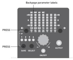
In Backpage mode, the first four columns of the display are used to edit four different parameters. Each parameter is denoted by a two letter abbreviation. They are as follows:
