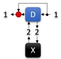
**External Loop Pre-Effect:** In this mode, an external effects pedal is inserted in series before the delay line, and it only becomes active when the Nemesis is activated. Connect the external effects pedal's input to Output 2 of the Nemesis, and connect the external effects pedal's output to Input 2 of the Nemesis.
