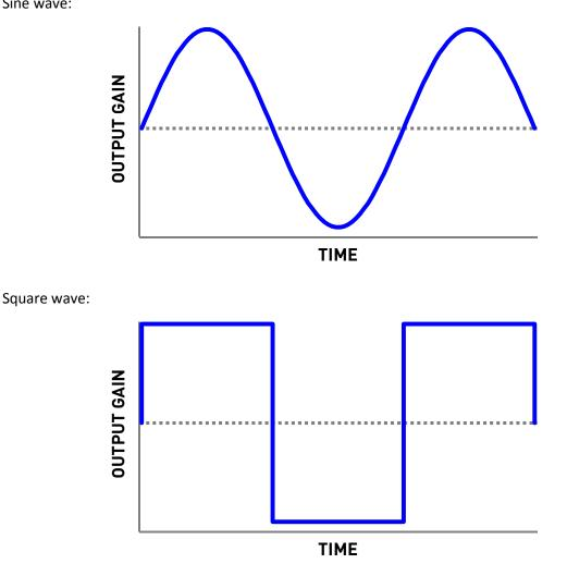
By default, the Mercury uses a sine wave for its LFO, but other wave shapes can be selected using the Neuro App.
