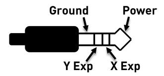
Third party expression pedals can be used as well, as long as they have a TRS (Tip Ring Sleeve) plug with power on the tip, expression (the wiper of the potentiometer) on the ring, and ground on the sleeve, as seen in the diagram below.
