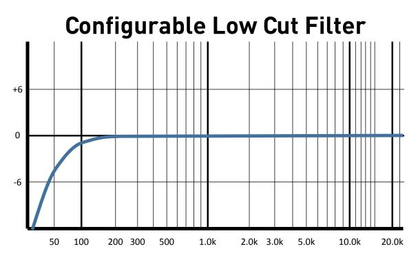
The Parametric EQ and the Low Cut filter are configurable using the Neuro App. By default, the parametric EQ is disabled (flat), and the Low Cut filter is set to 10 Hz.
