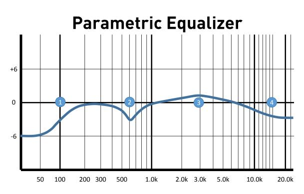
Using the Neuro App, Band 1 (Low Shelf) can optionally be configured as a high pass filter, and Band 2 (High Shelf) can optionally be configured as a low pass filter.
