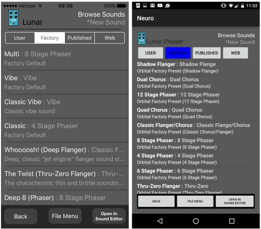
The Browse Sounds screen displays lists of presets that can be easily loaded into the hardware. Just tap on a preset name to send it to the hardware, and you should be able to hear it instantly.
