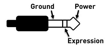
Expression pedals with TS (Tip Sleeve) plugs will not work correctly with the Lunar.
