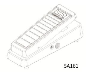
Thank you for purchasing the SA161 Dual Expression Pedal. This rugged, cast-aluminum expression pedal features two independent Expression Outputs as well as a Sensor Output for use with Source Audio Soundblox effects pedals. The dual TRS expression outputs allows the SA161 to control two Soundblox Pro (or other 3<sup>rd</sup>-party) units simultaneously.
