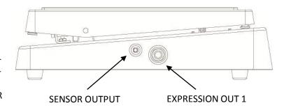
Note: Expression Output and Sensor Output can NOT be used simultaneously!
