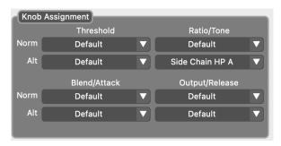
Many Source Audio pedals contain knob assignment (or re-assignment) controls for top-level flexibility. The Atlas is no different. Each of the top four knobs and each of the four ALT controls can be reassigned in this module from a list of parameters. The knob assignments are set and stored on a preset-by-preset rather than global basis for ultimate flexibility of control.
