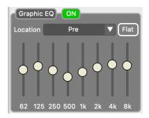
For ultimate tone-sculpting, we've included an 8-band graphic equalizer within the Atlas Compressor. The Graphic EQ can be switched on or off per preset. Additionally, the graphic EQ can be applied either before (Pre) or after (Post) using the "Location" dropdown menu.
