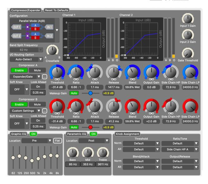
**Configuration**: Select how the Atlas's onboard compressors are configured within the signal path. Choose between the options below.
