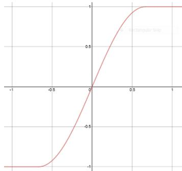
Bob's Notes: *"I think the soft corners are more characteristic of tubes than transistors or op-amps. It's missing the asymmetry between high and low clipping, and it doesn't attempt to match the 3/2 power law characteristic of tubes. But for only one word [for a description], best I can think of."*
