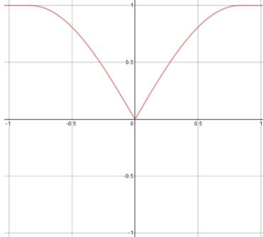
Bob's notes: *“If one puts a sine wave through a full wave rectifier, the output frequency is twice the input frequency. This is how we get an octave up. The full-wave rectifier (FWR) is used in all analog octavers.”*
