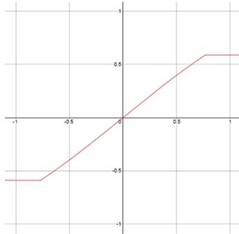
**Offset** – Similar to asymmetrical diode clipping found in analog overdrive/distortion pedals.
