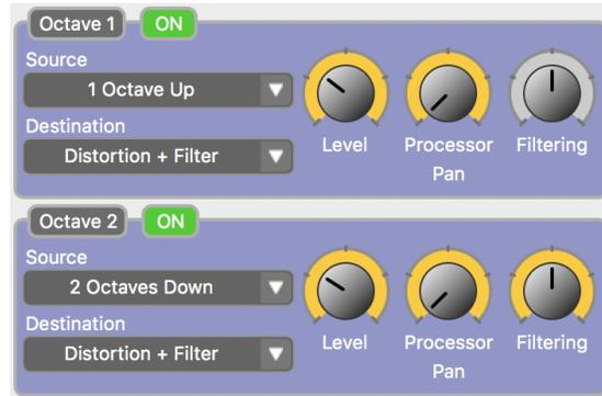
In addition to the two Standard Voices the Spectrum features two monophonic Octave Voices that can be added to the final mix. Each Octave Voice can be set either one octave up or up to two octaves down.
