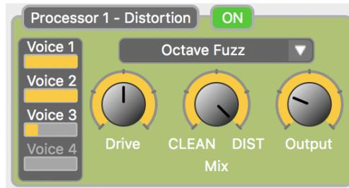
Adds distortion to any of the Standard or Octave Voices. The high harmonic content of added distortion will heavily accentuate the sound of the modulating filters. The Spectrum includes 13 types of distortion, anything from a subtle drive effect to extremely fuzzy Foldback effects.
