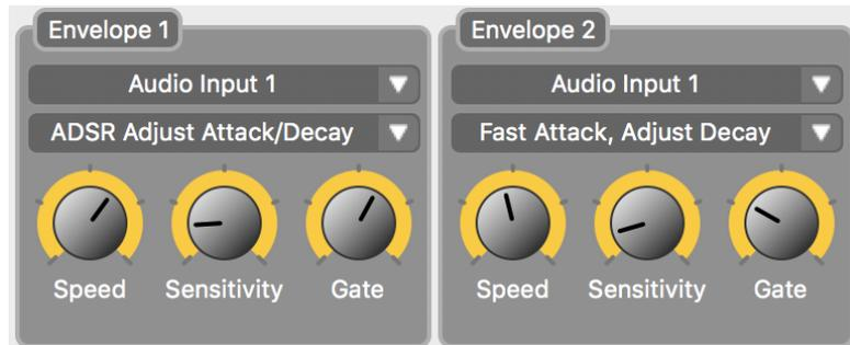
The Envelopes control amplitude and filter modulation of the each Spectrum Voice. Both Envelopes 1 and 2 run independently of each other and each can be assigned a different set of Voices.
